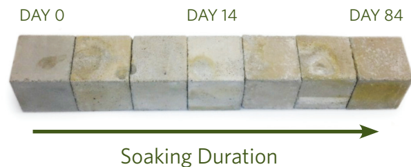
Figure 3. Cubes of the GeoSpray AMS system after soaking in 1% H_2SO_4
